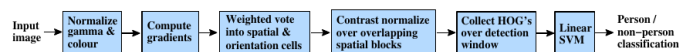
Fig. 1. Description of sequential processing stages for extracting HOG features and perform an image classification task; Image from [2].
