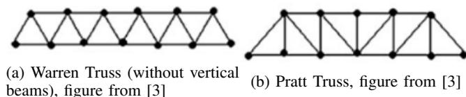
Fig. 1: Truss Types
