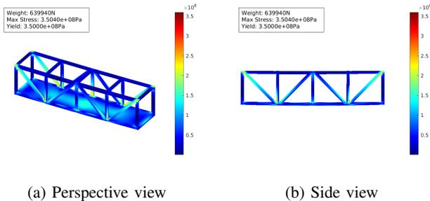
Fig. 8: Bridge model with diagonal trussing, with approximately 640kN of force applied to it.
