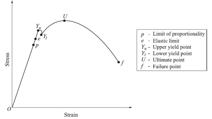
Fig. 3: Illustration of a stress-strain curve for ductile materials [5].
