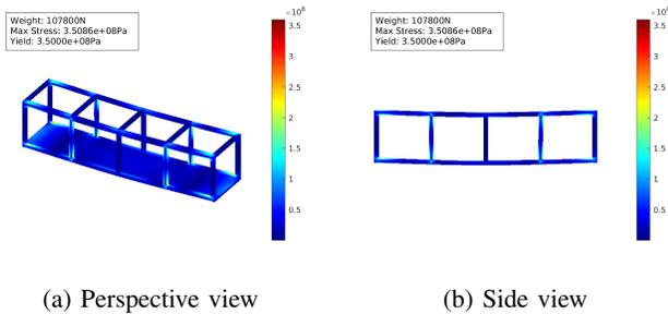
Fig. 7: Bridge model without diagonal trussing with approximately 108kN of force applied to it.
