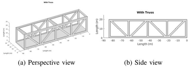
Fig. 4: Bridge Model with Diagonal Trussing
