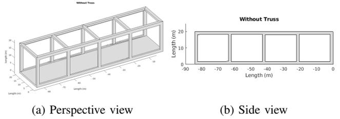
Fig. 5: Bridge Model without Diagonal Trussing
