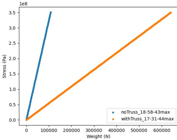
Fig. 6: Plot of the maximum stress of the structure over weight applied for both models.
