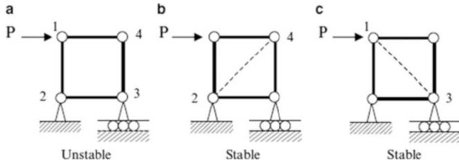
Fig. 2: Illustration of three structures with varied stability. Bottom left corner of each rectangle is fixed and bottom right corner is connected to a roller [3].
